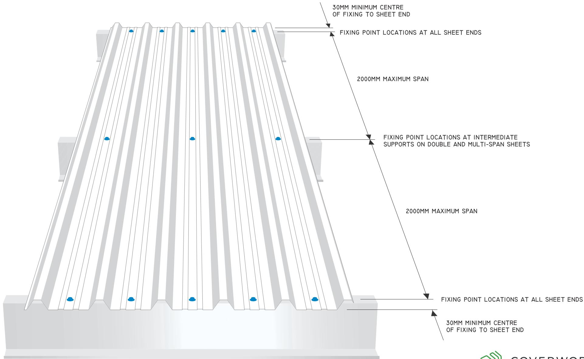
THIS ASSEMBLY USING THE 32/1000 PROFILE IN 0.7MM THICKNESS HAS BEEN IMPACT LOAD TESTED TO ACR(M)001:2019 (TEST FOR NON-FRAGILITY OF LARGE ELEMENT ROOFING ASSEMBLIES) AND ACHIEVED CLASS B NON-FRAGILITY RATING FOR SINGLE, DOUBLE AND MULTI-SPAN CONDITIONS.
